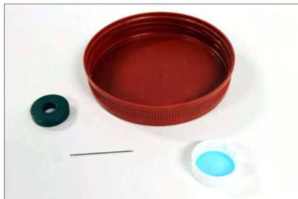
Materials to make one compass. Note: the magnet does not need to be a ring magnet—any magnet will work.
